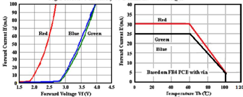
Fig.2 Forward Current vs Forward Voltage
