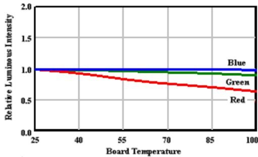
Fig.5 Luminous Intensity vs Board Temperature
