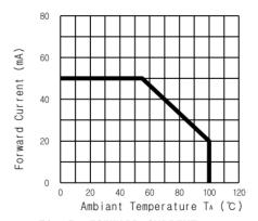
Fig.5 FORWARD CURRENT DERATING CURVE
