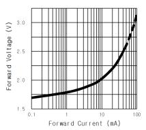
Fig. 3 FORWARD VOLTAGE V.S. FORWARD CURRENT
