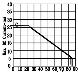
Fig5. MAX. ALLOWABLE DC CURRENT VS. AMBIENT TEMPERATURE.
