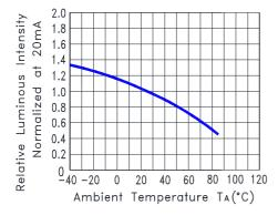
Fig.5 Relative Luminous Intensity vs. Ambient Temperature
