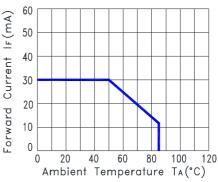
Fig.2 Forward Current Derating Curve
