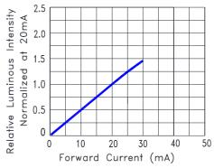
Fig.4 Relative Luminous Intensity vs. Forward Current
