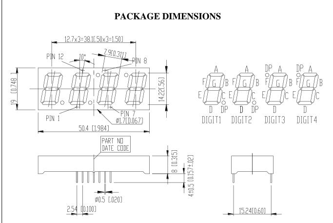
NOTES: 1. All dimensions are in millimeters. Tolerances are  $\pm$  0.25mm (0.01") unless otherwise noted. 2.Pin tip's shift tolerance is  $\pm$  0.4 mm.
