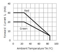
Fig. 3 FORWARD CURRENT VS. DERATING CURVE
