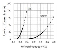
Fig. 2 FORWARD CURRENT VS. FORWARD VOLTAGE
