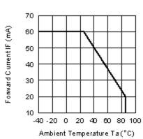
FIG.2 FORWARD CURRENT VS. AMBIENT TEMPERATURE
