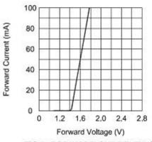
FIG.3 FORWARD CURRENT VS. FORWARD VOLTAGE
