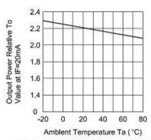
FIG.4 RELATIVE RADIANT INTENSITY VS. AMBIENT TEMPERATURE
