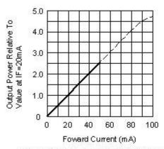
FIG.5 RELATIVE RADIANT INTENSITY VS. FORWARD CURRENT
