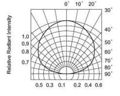
FIG.6 RADIATION DIAGRAM
