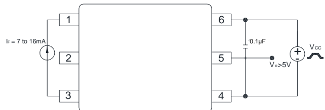
Figure 19 : UVLO Test Circuit
