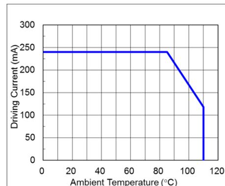
Fig 5. FORWARD CURRENT DERATING CURVE
